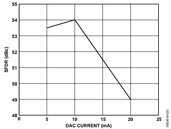
Figure 20. SFDR vs. DAC Current, 59.1 A OUT , 300 MHz REFCLK with REFCLK Multiplier Bypassed
